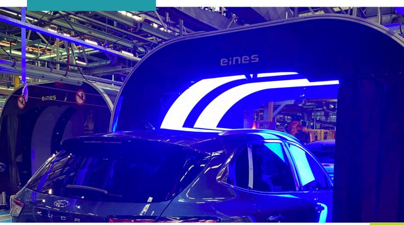
Eines Inline Flush & Gap inspection system
